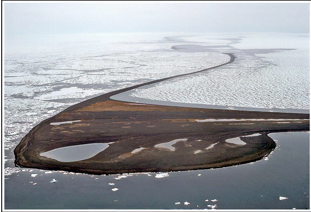
View looking east at Point Barrow on the Alaska North Slope in late July 1976. This is a classic example of a cusped foreland formed by opposing significant wave directions, in this case from the east and the west. Note that ice was still covering much of the surface of the Arctic Ocean in that particular area.
